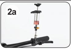
For levers and calipers with bleed ports on the top, use the upright syringe clip (E).
