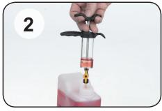
Use the plunger to draw brake fluid into the syringe.
