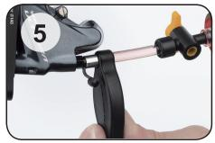
Attach the adapter hose to the bleed nipple on the caliper, then press the hose bushing (J) onto the nipple using the hose holder (G) to secure it.
