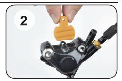
Remove the brake pads from the caliper and insert the bleed block before bleeding. Secure in place with the pad axle.
