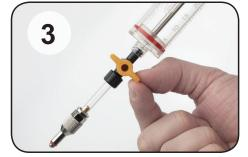
Turn the lever on the valve clockwise to close the system and prevent fluid from entering or leaving the syringe. Once ready to bleed the brakes, turn the lever counterclockwise to open the system.
