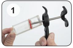
The plunger can be removed from the syringe (A) for cleaning. Unscrew the handle, then pull the plunger to remove. Dry all parts thoroughly before performing another bleed.
